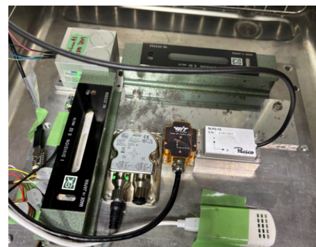
Fig 2. A system to evaluate the tilt sensors.
