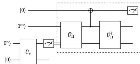
Figure 1. Quantum circuit for estimating the persistent Betti numbers.  $\tilde{U}_s$  is a unitary for state preparation and  $\tilde{U}_\Pi$  is a unitary encoding of the projector onto the ground space of the persistent Laplacian.
