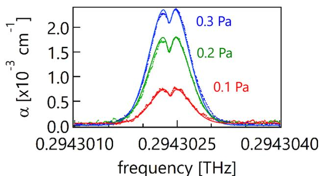
Fig. 1: Pressure dependence of the absorption spectrum of  $(J, K) = (15, 0) \rightarrow (16, 0)$  rotational transition in acetonitrile under THz pumping in several pressures. dots: measured data, lines: fitting curves.
