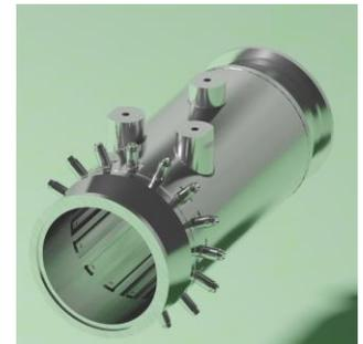
Fig. 1. 3D model of the 16-electrode beam monitor
