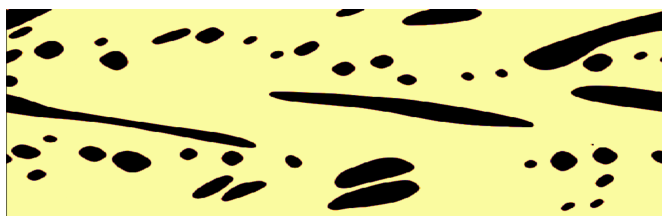
Fig. 2. A typical snapshot of the channel-like structures. yellow: liquid phase, black: gas phase
