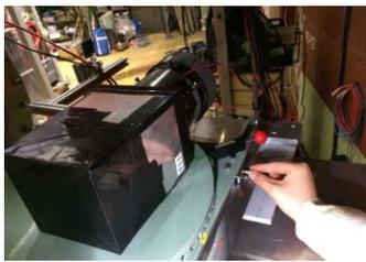
Fig.1 A module of the lead-glass calorimeter.
