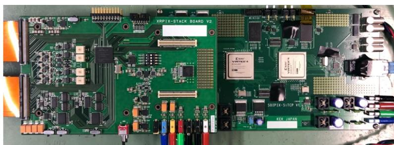
Fig. 2. Data acquisition system.
