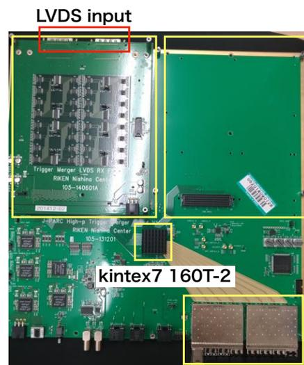
Fig. 2: trigger merging module (P+)
