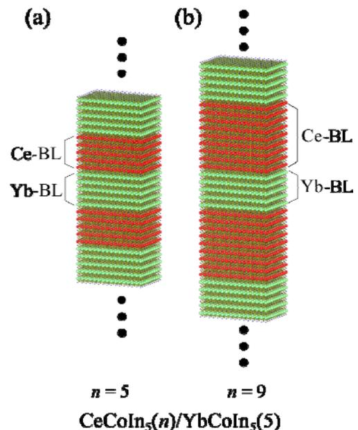
Fig. 1 The schematic image of the superlattices of  $\text{CeCoIn}_5(n)/\text{YbCoIn}_5(5)$ . The BLs of  $n$ -unit cell thick  $\text{CeCoIn}_5$  and 5-unit cell thick  $\text{YbCoIn}_5$  are stacked alternately. The set of Ce-BL and Yb-BL repeats several times.
