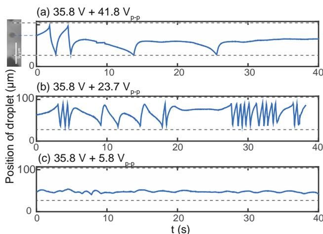
Fig. 1 Time Evolution of the droplet position. The voltage from the amplifier is (a)  $35.8 \text{ V} + 41.8 \text{ V}_{\text{p-p}}$ , (b)  $35.8 \text{ V} + 23.7 \text{ V}_{\text{p-p}}$ , (c)  $35.8 \text{ V} + 5.8 \text{ V}_{\text{p-p}}$ . The position of the droplet was measured along the line between the electrodes. The position of electrodes is about 100 and 20  $\mu\text{m}$  (the dashed lines).
