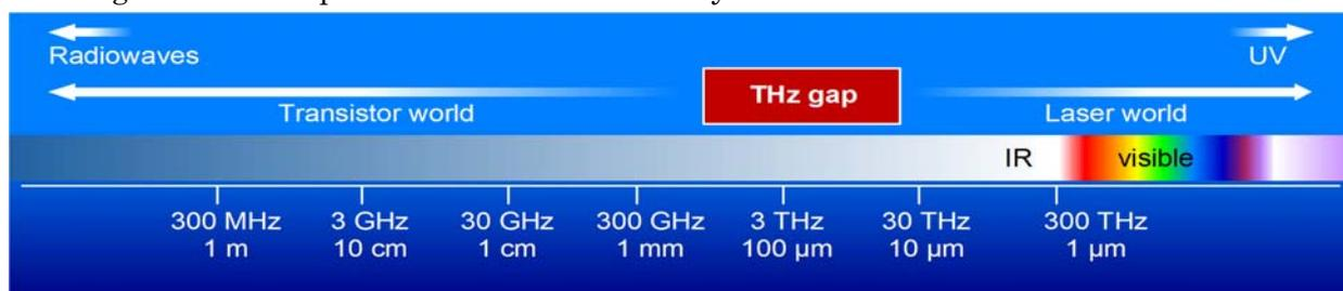
Fig. 1: Illustration of the electromagnetic spectrum showing the terahertz region between the longer electronic wavelength and the shorter optical wavelengths, also called the terahertz gap.
