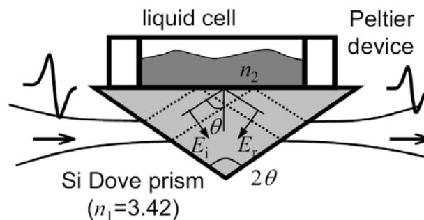
*Fig. 3: Principle of ATR on liquids with temperature control*
