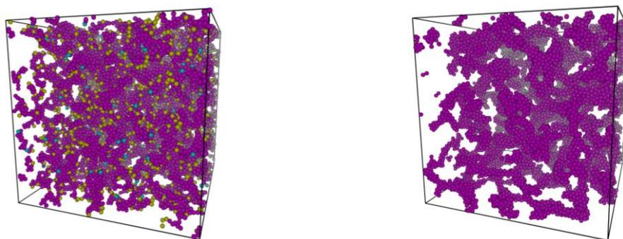
Fig. 1. Snapshots of two type colloidal gels (volume fraction = 6%). Left: MD-DLCA model. Right: S model. Coloring depends on the number of adjacent particles(N). N=1 is cyan, N=2 is yellow and  $N \geq 3$  is purple.
