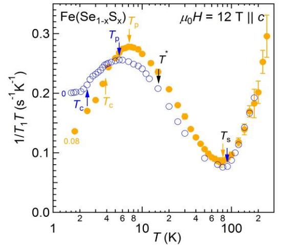
Fig. 1. Temperature dependence of  $(T_1T)^{-1}$  on  $\text{Fe}(\text{Se}_{1-x}\text{S}_x)$  ( $x = 0, 0.08$ ) in  $\mu_0H = 12$  T.
