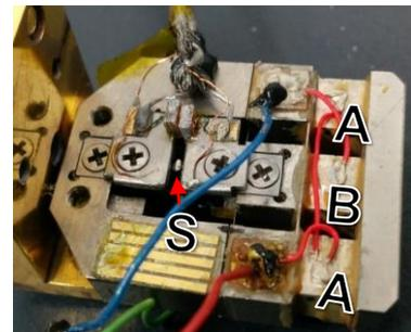
Fig. 1. Strain applying device with a sample (S) attached to a holder to be mounted in the vector magnet. The two outer (A) and one inner (B) piezoelectric elements apply tensile and compressive strain, respectively.
