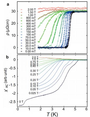
**Figure 1** (a) Resistivity  $\rho$  and (b) Real part of AC susceptibility  $\chi'_{AC}$  as a function of temperature of  $\text{Sr}_{3-x}\text{SnO}$  under zero and various magnetic fields. The  $\chi'_{AC}$  measurement under 0 T is cooled down to  $\sim 0.15$  K [4].
