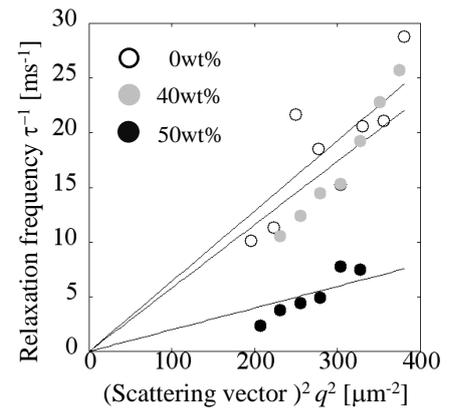
Fig.1. Dispersion relations for the twist mode of C-director in the pure and swollen SmC phases.
