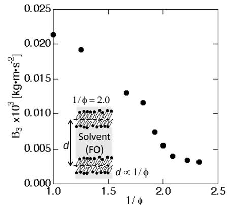
Fig.2. The dependence of  $B_3$  on the inverse of the volume fraction of BI with respect to the perfluorinated oil.
